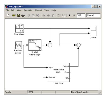
The positive input to the second Sum block is the sum of the input signal and the low frequency noise, s(n) + y. The negative input to the second Sum block is the LMS Filter block's best estimation of the low frequency noise, y'. When you subtract the two signals, you are left with an approximation of the input signal.
