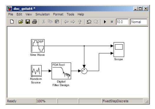
**3** Run your model and view the results in the Scope window. This window shows the original input signal and the signal with low frequency noise added to it.
